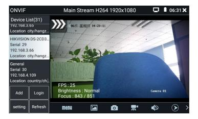
**IP camera video settings:** Click "Video Set" to enter the main stream setting interface of webcam video make the required changes and click OK to save. The main stream parameters inside the webcam change as well.
