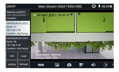
Some network cameras may not scan automatically, you can manually add the camera. Tap "Add" in the bottom left and users can manually add a camera. Click "Refresh" and the tester scans the ONVIF network camera again. Click on the device
