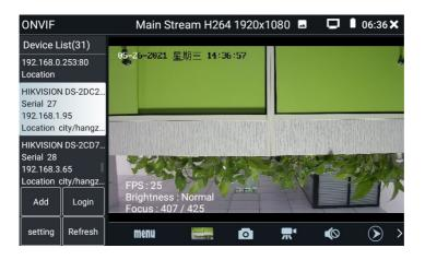
**Snapshot:** Click bottom "snapshot" icon to get the currently displayed image and generate a photo, store in the internal storage or external SD card.
